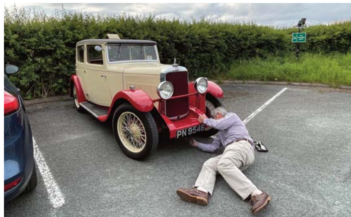
June's meeting saw Pater Lakin checking axle fixings in an attempt to cure some wayward steering
